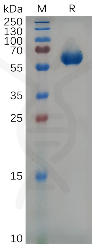
Figure 1. Mouse CS1 Protein, hFc Tag on SDS-PAGE under reducing condition.
