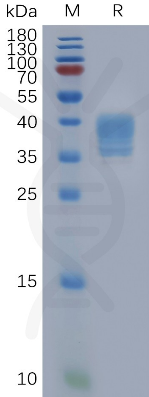
Figure 1. Human F2RL1 Protein, hFc Tag on SDS-PAGE under reducing condition.
