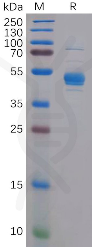
Figure 1. Human CLEC2D Protein, hFc Tag on SDS-PAGE under reducing condition.
