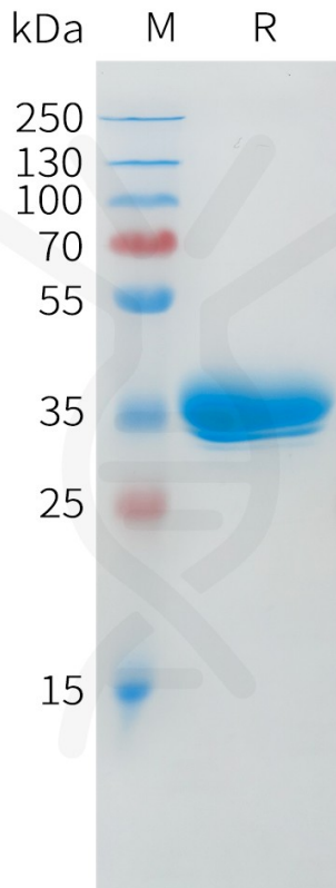
Figure 1. Cynomolgus BCMA Protein, hFc Tag on SDS-PAGE under reducing condition.
